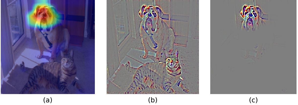
Figure 2 – Prediction: Dog; explanations produced by (a) CAM, (b) GBP, and (c) Guided GradCAM. Source: (Selvaraju et al., 2017).
