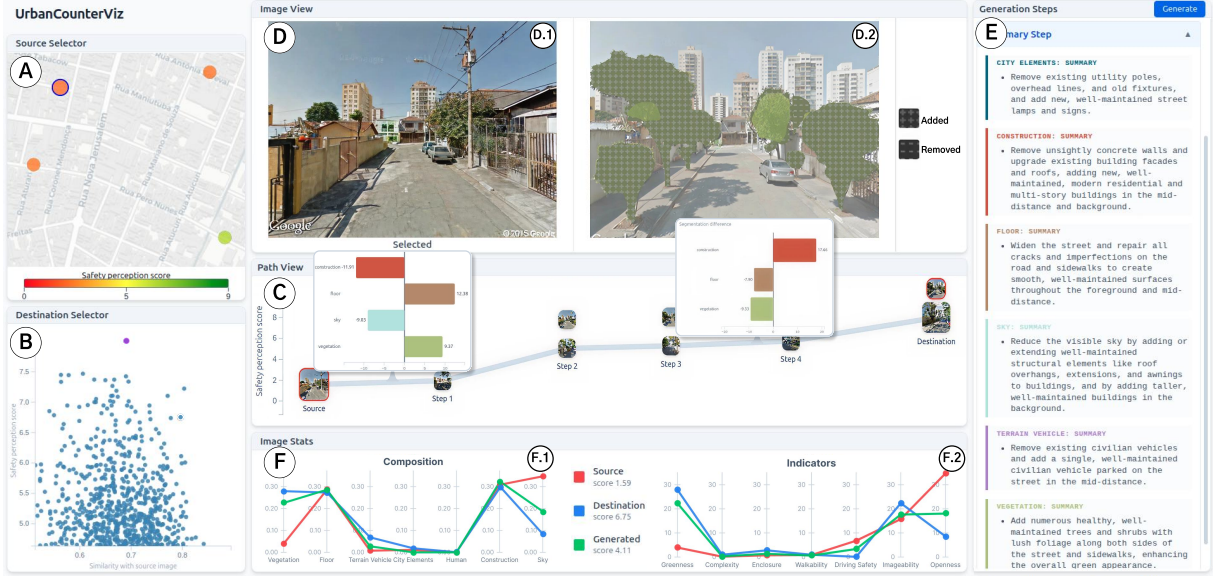
Figure 21 – URBANCOUNTERVIZ interface. (A) Source Selector : geo-located images colored by perceptual Q-score; selecting a source initializes the workflow. (B) Destination Selector : scatterplot of candidate images showing visual similarity to the source (x) versus Q-score (y), supporting destination selection. (C) Path View : shortest path in the similarity graph from source to destination, exposing intermediate scenes and their semantic differences. (D) Image View : side-by-side comparison of the source (D.1) and generated counterfactual (D.2), augmented with overlays highlighting added and removed regions. (E) Generation View : stepwise editing actions organized by semantic category, enabling inspection of the generation process. (F) Image Stats : coordinated summaries comparing semantic composition (F.1) and urban indicators (F.2) across the source, destination, and generated images. Source: the author.
